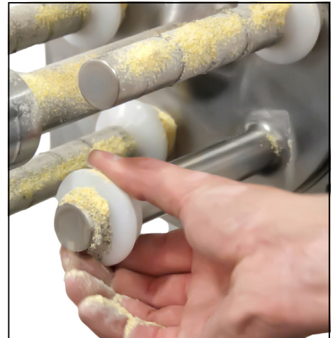
Magnets are cleaned completely outside the product zone with wiper rings.
