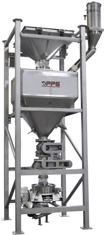
Piercing Bulk Bag Unloader with Integral Dust Collection, Surge Hopper, Rotary Valve, Delumper, & Sifter
